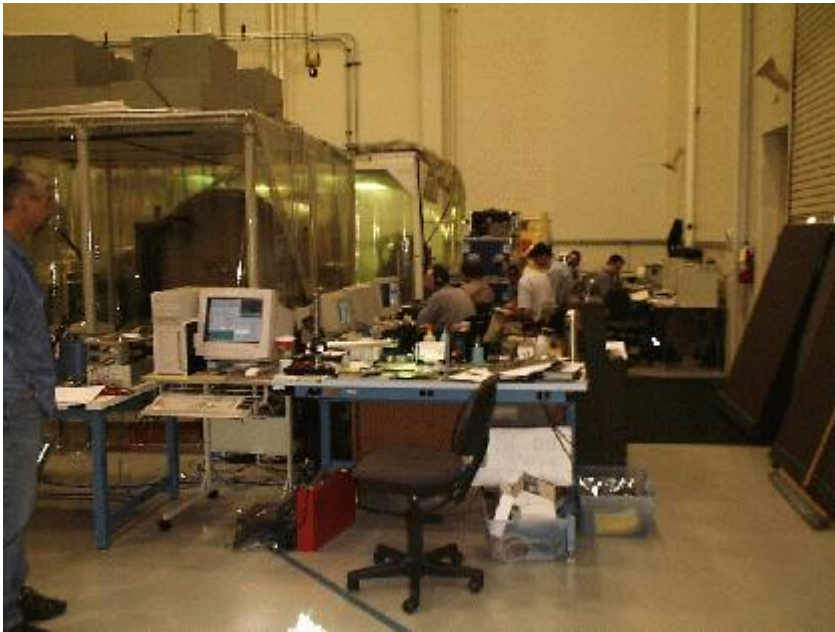
Figure 1. The high bay at SDL. The SABER test chamber is under a clean tent on the left. To the center and right are engineers operating the instrument during calibration tests. The computers mentioned in this article are along the right wall.
